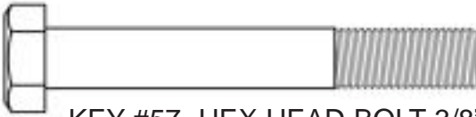
KEY #57 HEX HEAD BOLT 3/8" X 2 1/2" PARTIAL THREAD QTY. 1
