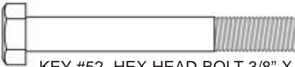
KEY #52 HEX HEAD BOLT 3/8" X 2 3/4" PARTIAL THREAD QTY. 4
