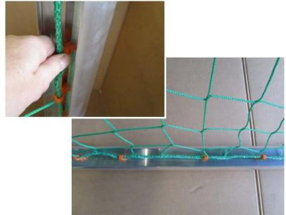
c) Fix the end of the enclosed cord in one ring nut and knot it well. Pull the cord through the net meshes and fix it at the top in the 2nd ring nut and knot it well.
