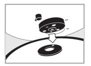
Position the magnetic wheel onto the magnetic adaptor on the projector.
