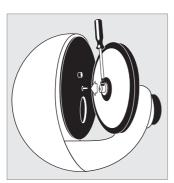
To attach glass bossed effect wheels such as liquid wheels, tighten the cross headed screw on the shaft of the wheel rotator as per the image left.
