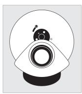
The [OPTI] Aura has been designed to accommodate 4" and 6" effect wheels. For 6" effect wheels the slide on the left of the magnetic adaptor should be at the top as per the image left.
