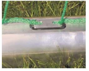
b) Now the tensioning cord can be tightened between the ring nuts which are provided at the net hoops.
