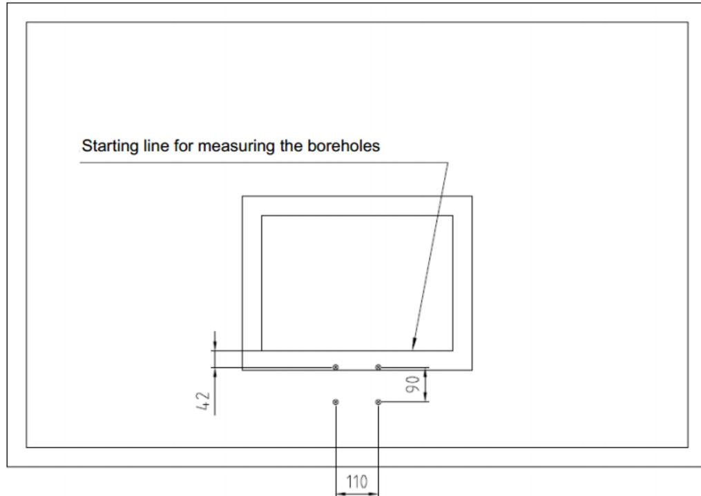
Figure 5: Borehole dimensions
