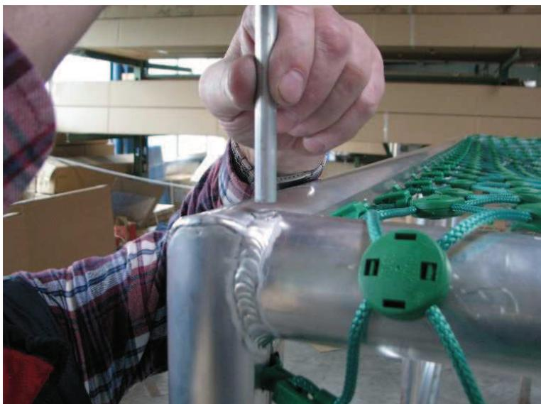
With the last two rods you safe the net from stealing. The end of this two rods is hard to put in with the hand, because of the tension from the net. Please use a piece of wood and a hammer therefor.
