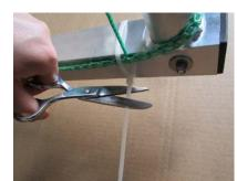
Fix net at the bottom of net hoops with 3 cable clips.Cut projecting parts.
