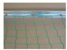
After having mounted all net holders fix net at the goal construction. Stick net holders in the net hook rail and fix them with a 90 degrees' rotation. In case, use for this a thin screw driver.
