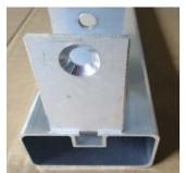
c) To fix the lower hinge stick from the bottom (upright's end) 1 nut 20 mm, M 8 each in the guide rail of the upright. Mount lower hinge with 1 fastening borehole. Please consider that the inclined side of the hinge points to the goal inside. Push nut 20 mm, M 8 below the borehole of the hinge and fix it at the upright with safety hexagon screw DIN 7991, M 8 x 16.
