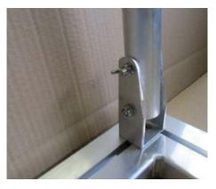
h) Press net hoop to the outside. Stick from the top hexagonal screw DIN 933, M 8 x 60 through the 2nd borehole of the upper hinge and the hoop. Then add washer DIN 125, Ø 8.4 mm at the hinge lower side and screw wing nut DIN 315, M 8.
