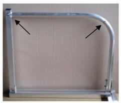
Stick ring nuts M 6 x 50 through boreholes of the net hoop (position see picture below) and fix them with washer DIN 9021, 7.4 x 22 and self-locking cap nut DIN 986, M 6.
