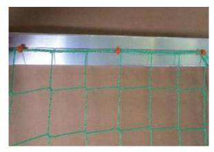
d) Fix one end of the attached cord in one of the ring nuts and knot it well. Pull the cord through the net meshes, fix it in the 2nd ring nut and knot it well. Cut the projecting part of the cord.
