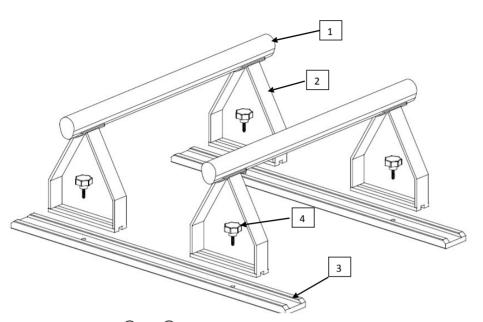
The bars and brackets ① and ② come pre-assembled. For assembly, put them on the wooden rails ③ as shown in the illustration. Fix the bar brackets to the wooden rails at the desired distance using the star grip screws ④.
