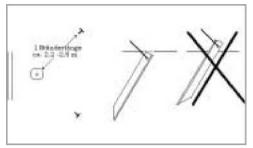
4. Place the posts next to the ground plate. Hammer the pegs approx. one post section length from the ground plate and roughly as shown into the ground. Hammer the pegs completely into the ground to prevent injuries from protruding parts. Only completely sunk pegs guarantee optimum anchoring.
