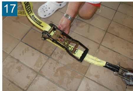
17 Connect slackline with ratchet
