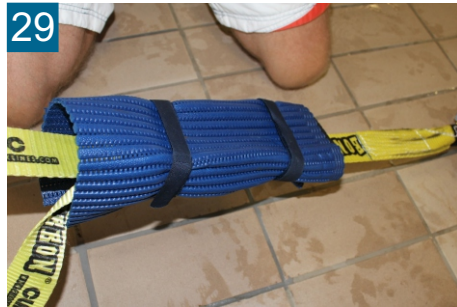
Fix ratchet cover with velcro fastener
