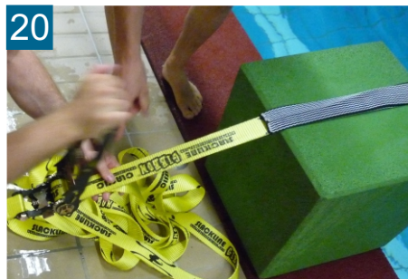
20 Tighten by tension and use ratchet (3 turns) before line grips
