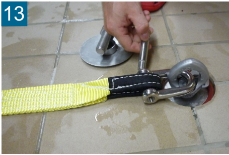
13 Connect fixing screw and slackline with shackle
